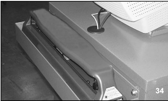
30. Store body scanner in body scanner tray at rear of workstation. (Figure 34.)
