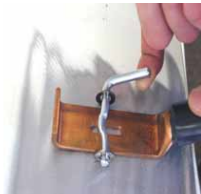
Fig. 29: Copper shoe and lever clamp
