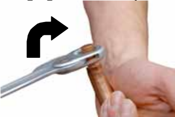
Fig.32: Exchanging electrode caps
