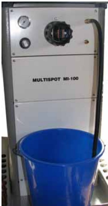
Fig.57: Draining cooling water.
