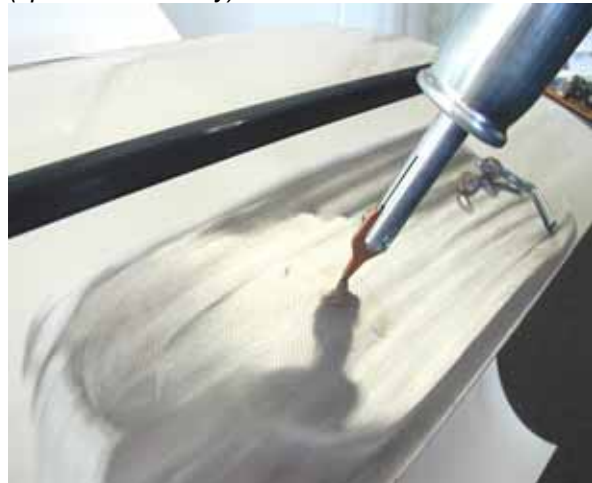
Fig. 45: High speed planishing hammer, SAH' (special accessory)
