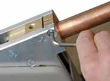
Fig.30: Unbolting electrode arm
