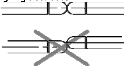
Fig.36: "Electrode must be in true alignment"
