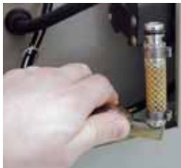
Fig. 56: Water filter loosened
