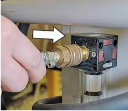
Fig.24: Connecting compressed-air supply
