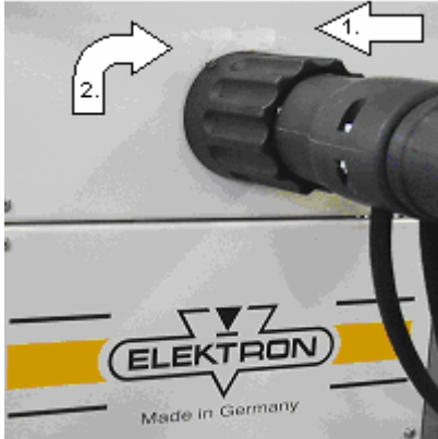
Fig. 28. Connecting the gun
