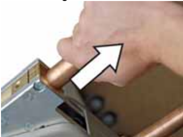
Fig.31: Removing the electrode arm.
