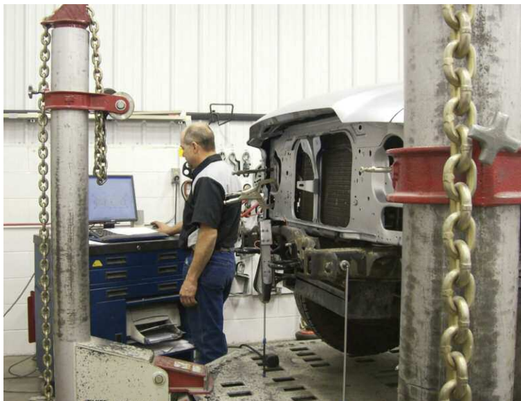
Lefler Auto Body Tech Rodney Blandford works on a vehicle using the shop's Chief Impulse frame rack, one of the Chief machines that Lefler counts on to repair approximately 200 cars weekly
